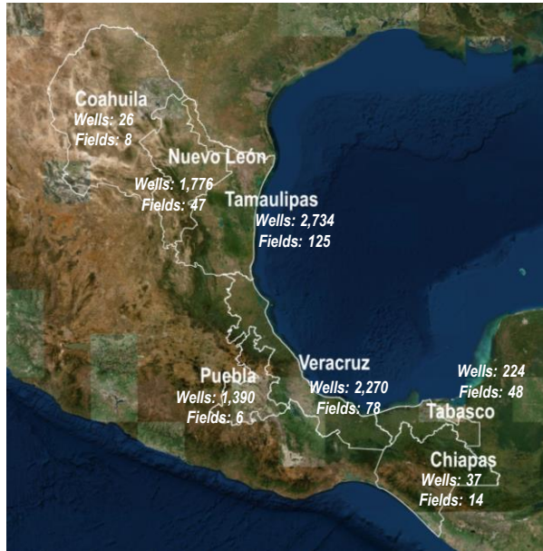
Number of wells utilizing hydraulic fracturing and the number of fields where they are located
